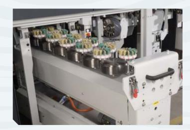
The bottom sanding stations are arranged vertically and therefore easily available for a sanding belt change. The belt lengths of the bottom sanding stations are identical with the belt lengths of the top sanding stations.
