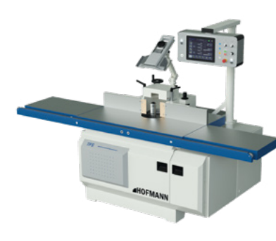
TF / TFS 1245 in version with CNC control here with table 2.7 m
