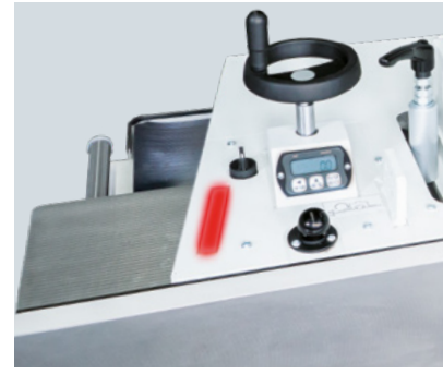
Safety light bar at the fence
