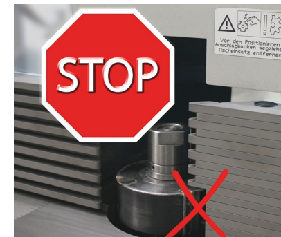
Guardian (the clamping of the fence jaws is monitored)
