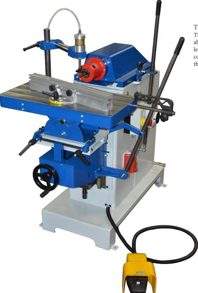
PEDAL POCKET LOCKING The pneumatic clamping of the pedal makes the loading and unloading of the pieces convenient and quick, ensuring an optimal fixing during the processing.
