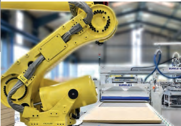
Roboterbestückung mittel Vakkumtraverse Robot loading with a vacuum traverse
