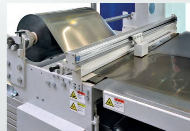
Abwickelstation um Rollen- in Bogenware zu schneiden. Cutting device to cut coils to sheet.
